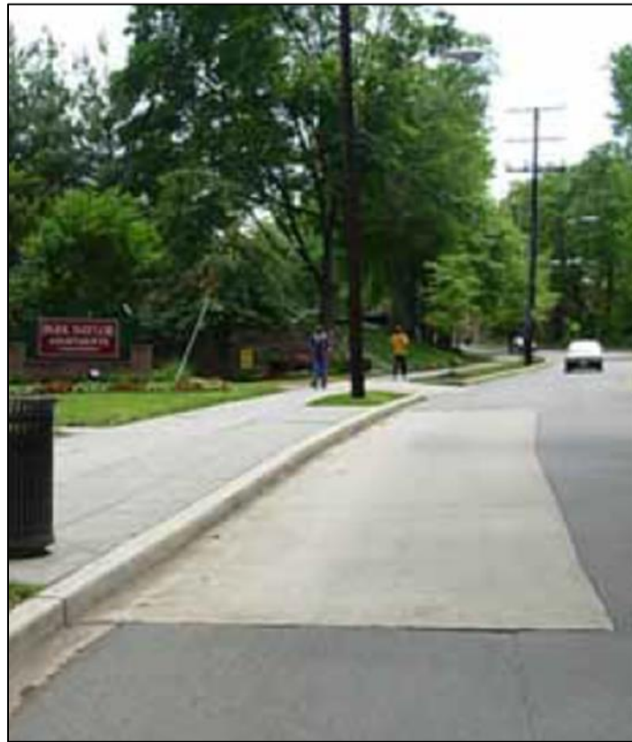
Figure 31: Example of Concrete Bus Pad
