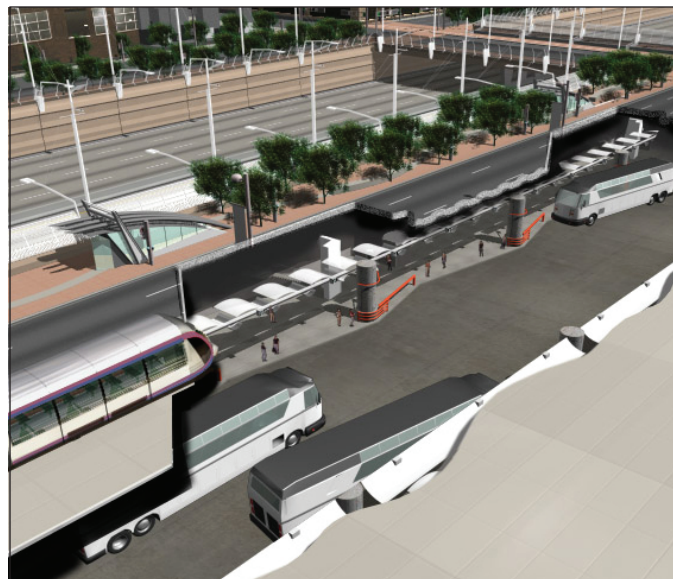
Cut-away rendering of the Riverfront Transit Center, with buses in the tunnel and light rail above on Second Street.
